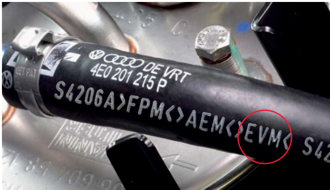
Figure 11: Flame-retardant and chlorine-free fuel hose cover made of Levapren ® by Veritas**
