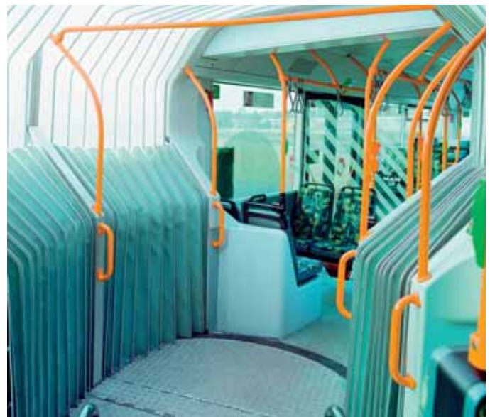
Figure 26: Vitroflex® made of Levapren® (© ContiTech AG)
