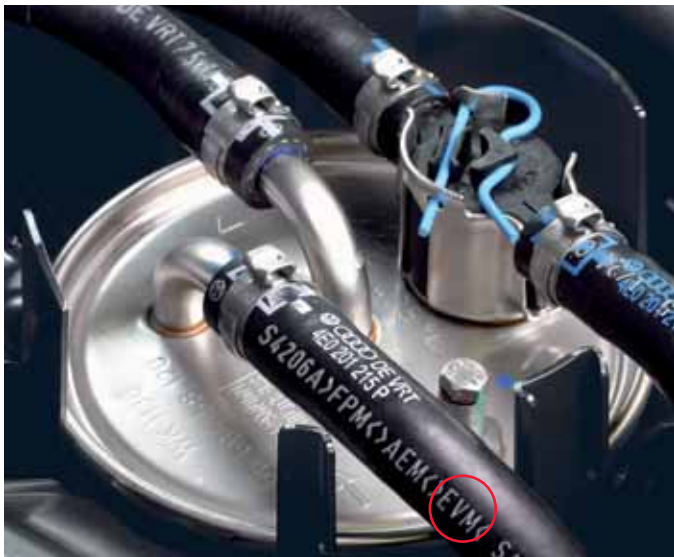
Figure 21: Flame-retardant and chlorine-free fuel hose cover made of Levapren®
